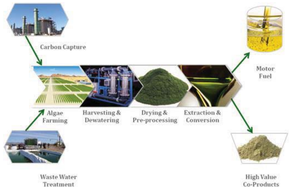
FIGURE 14 | Process of Growing Algae for Fuel. ASU Laboratory for Algae Research and Biotechnology
