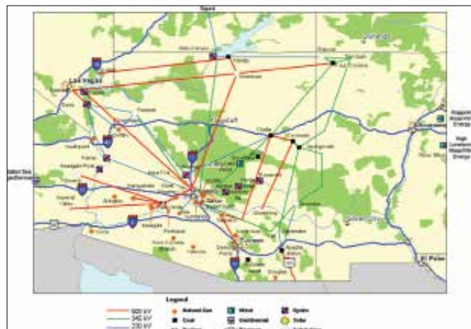
FIGURE 9 | Generalized Map of Transmission and Electric Generating Stations Supplying Power to Arizona
